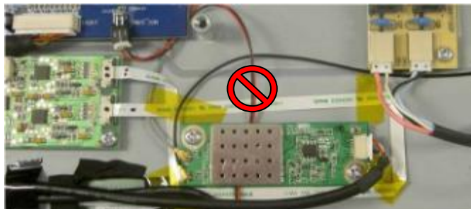
Figure 22: Example of how not to route FFC
